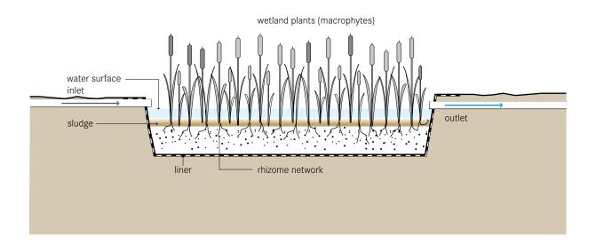
A free-water surface constructed wetland aims to replicate the naturally occurring processes of a natural wetland, marsh or swamp. As water slowly flows through the wetland, particles settle, pathogens are destroyed, and organisms and plants utilize the nutrients. This type of constructed wetland is commonly used as an advanced treatment after secondary or tertiary treatment processes.
